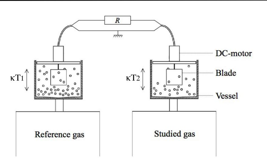
Fig.1: Sketch of the experimental setup: granular gas of ~350 steel beads of 0.1mg, 3mm diameter, accelerated independently at a few g by 2 shakers. 2cm blades are embedded in each gas, free to rotate about a vertical axis. Their rotational motion is detected by reversible DC micro-motors.
