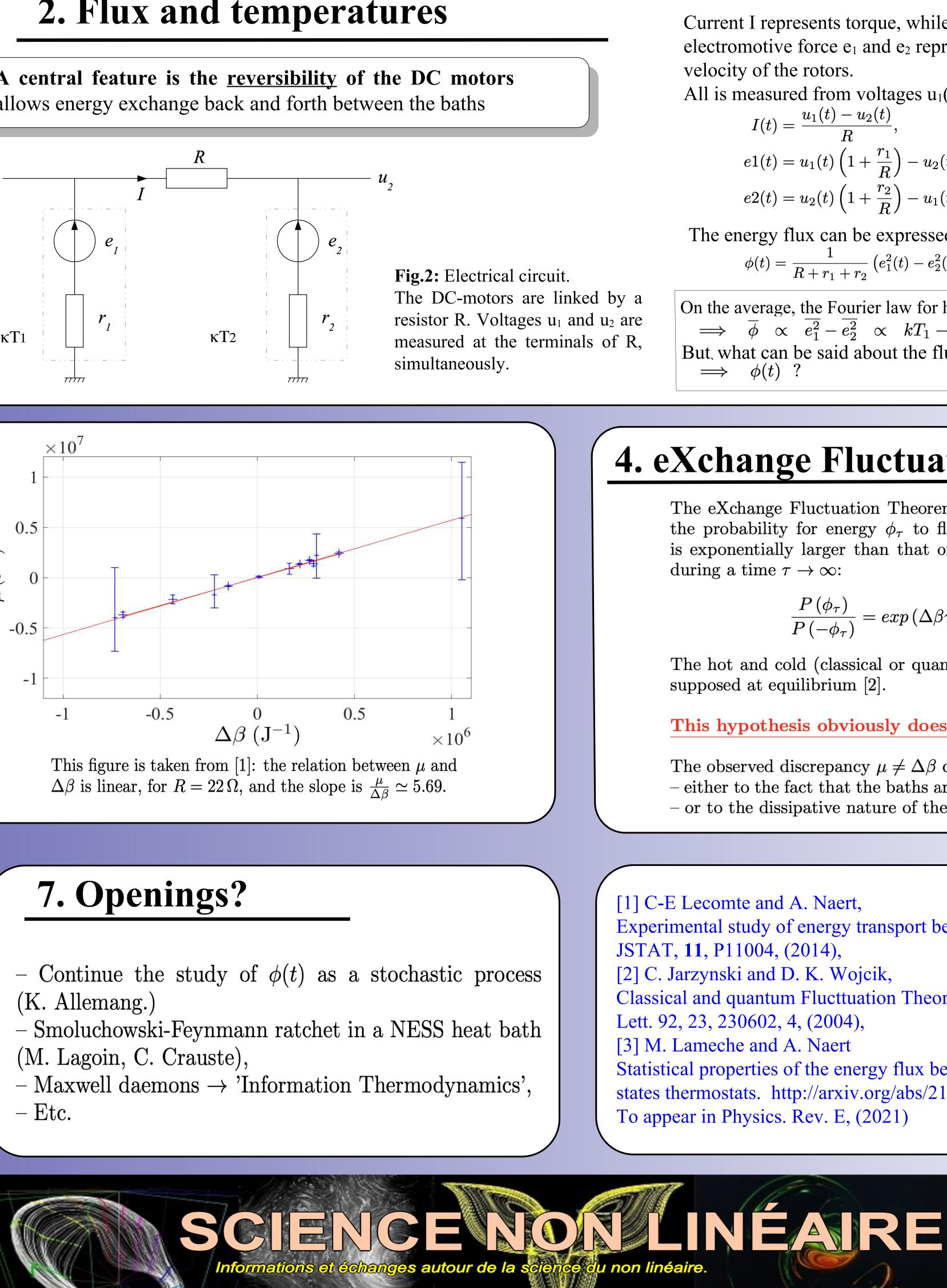
This experiment allows to investigate in a simplified configuration the relation between energy flux and temperature gradients in generic dissipative driven systems. It consists of two stationary granular gas thermostats excited separately in Non-Equilibrium Steady States (NESS), at distinct temperature, coupled in such a way that energy can flow between them.
