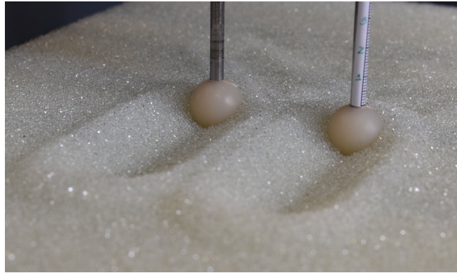
Figure 1. Two spheres (20 mm in diameter) moving side-by-side close to the surface of a granular medium.
