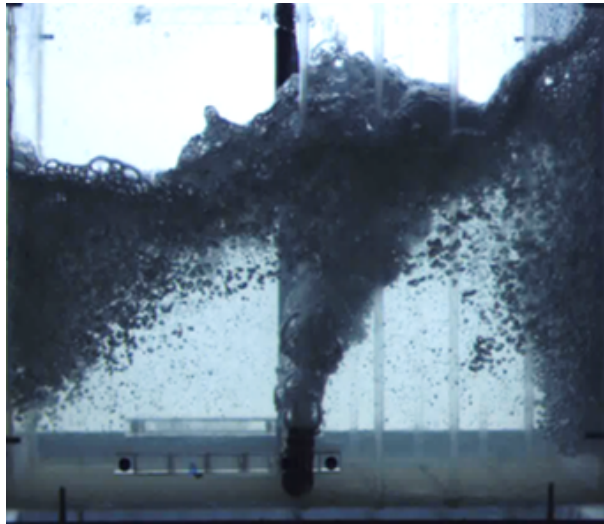
Figure 1. Planar view of the bubble plume with self-induced sloshing
